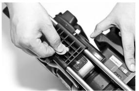
3. Insert the L-bracket slide (ML-SL30 or ML-SL15) into the hole of the Tripod Adapter and tighten the fastening screw. Hook the battery on to the slide and connect it to the light with the power cable (ML-PC1).
